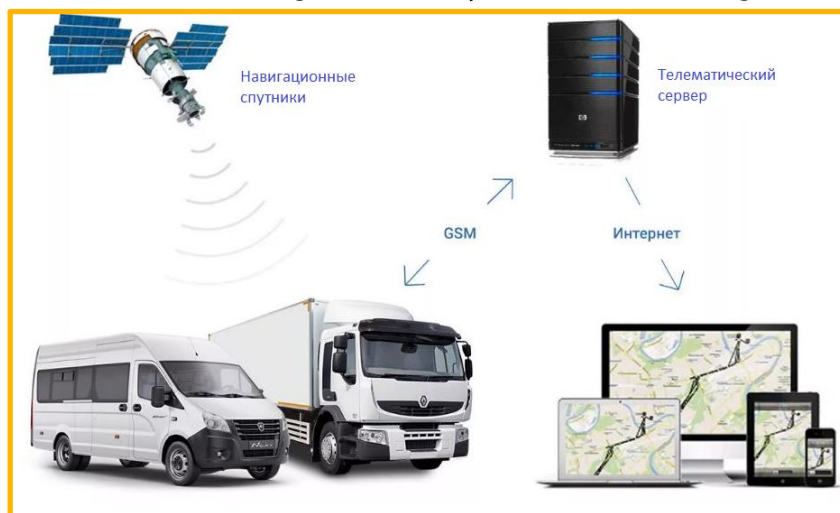
Figure 4: Structure of the monitoring and control system for vehicles using GNSS technologies.
