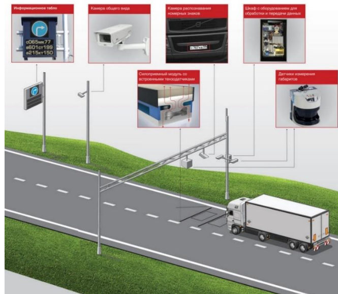
Figure 11: . Example of a modern station of weight and dimensional control and its equipment.
